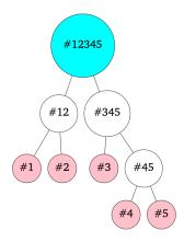
Let  $d_i$  be the distance from the leaf that denotes ingredients to the root (the number of edges between them), then the value of the final ingredients will be  $v_1/2^{d_1} + \ldots + v_N/2^{d_N}$ . To obtain the maximum result, you only have to think about the composition process such that  $d_1 \leq d_2 \leq \ldots \leq d_N$  (otherwise, you can swap some indices of ingredients so that the total result will increase).
